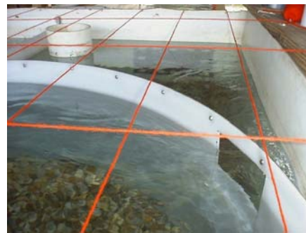
Figure 51. Habitat map of raceway. OS= outside straight-away, IS= inside straight-away, OM= outside meander, MC= mid-channel, BW= backwater
