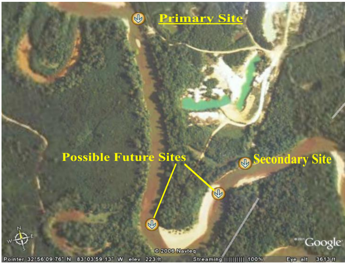
This picture shows the primary site selected for gravel augmentation (the existing gravel bar), a secondary site and possible future sites in the Oconee River. GADNR Photo
