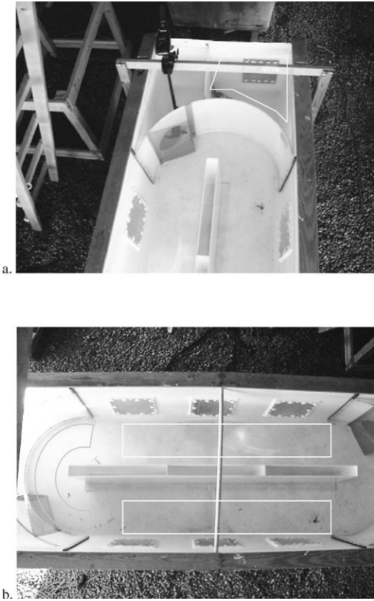
FIGURE 1.—Panel (a) shows a top view of the mesocosm in which the habitat preferences of robust redhorses were studied. The backwater environment, located in the upper right-hand corner behind the parabolic-shaped polyurethane divider, is outlined. Access to the backwater is via a window in upper right corner of the bend. Panel (b) shows a top view of the mesocosm with the main-channel environments and meander bend outlined (rectangles and semicircle, respectively).
