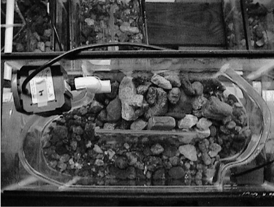
FIGURE 1.—Top view of aquarium modified to simulate pulsed, high-velocity water ( $>35$  cm/s) and stable, low-velocity water ( $<10$  cm/s). Water pumps were placed in squared pockets to prevent the eggs and larvae from being sucked into the water intakes.
